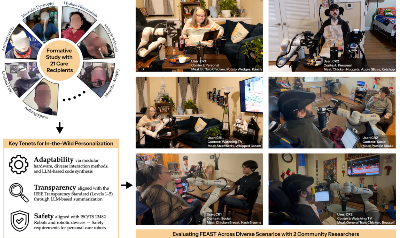
Fig. 1: Informed by a formative study with 19 care recipients and 2 community researchers, we propose FEAST: a flexible mealtime-assistance system grounded in adaptability, transparency, and safety. Through in-home evaluations, we demonstrate that FEAST can personalize to the needs of two care recipients, assisting each with three meals in diverse in-the-wild contexts.
