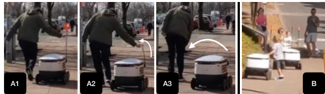
Figure 4: A: Pedestrian grabs the antenna and pulls it (Kingsley Park [00:04:11–00:04:21]). B: Children block the robots’ way as they inspect them excitedly (Leaving Coop [00:02:45–00:06:00]).
