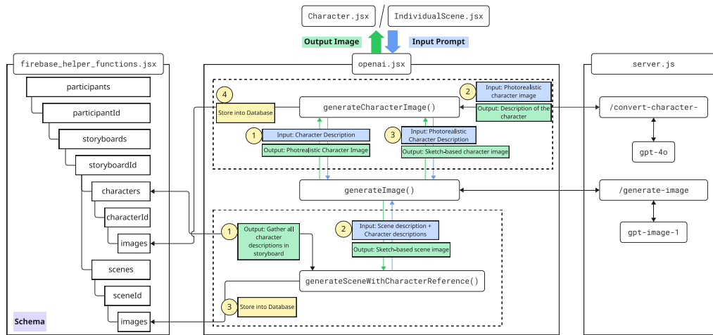
Fig. 2. SPEAK2SCENE backend workflow to generate images using OpenAI APIs. After receiving an input prompt, based on the function call ( generateCharacterImage() or generateSceneWithCharacterReference() ), the functions respectively interact with the Firebase database through functions defined in firebase_helper_functions.jsx and they interact with OpenAI API through server.js .
