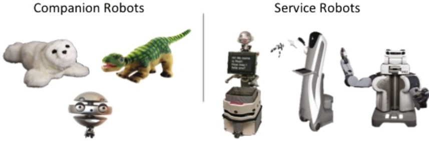
Fig. 1. Companion Robots (from left to right): Paro, Pleo, Emys; Service robots: Pearl, Care-O-bot, PR2. Categorization of assistive robots for older adults [4].
