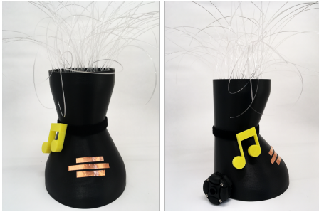
Figure 1: Perspectives of YOLO. From top to the bottom: transparent optical fibers; neck features velcro strip to attach toys of interest (e.g., a musical note was attached); 3 copper strips to sense touch; omni wheels for navigation.
