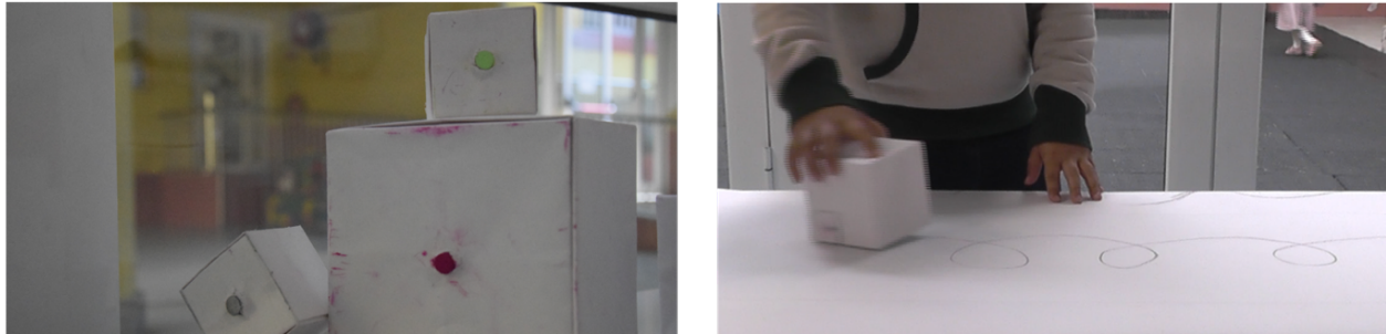
Figure 16. On the left: Paper prototypes of robots used in the design condition were made using origami techniques and each cube was built with a mechanism that integrates a crayon inside so that children could represent the movements of the robot by drawing them in large paper sheets. We embed a crayon in one of the cube faces as a design methodology that motivated children to represent the robot's movements in a 2D space, avoiding movements in a 3D plane (such as flying and jumping) as real robots are not able to do so. On the right: Example of a trajectory performed by a child.
