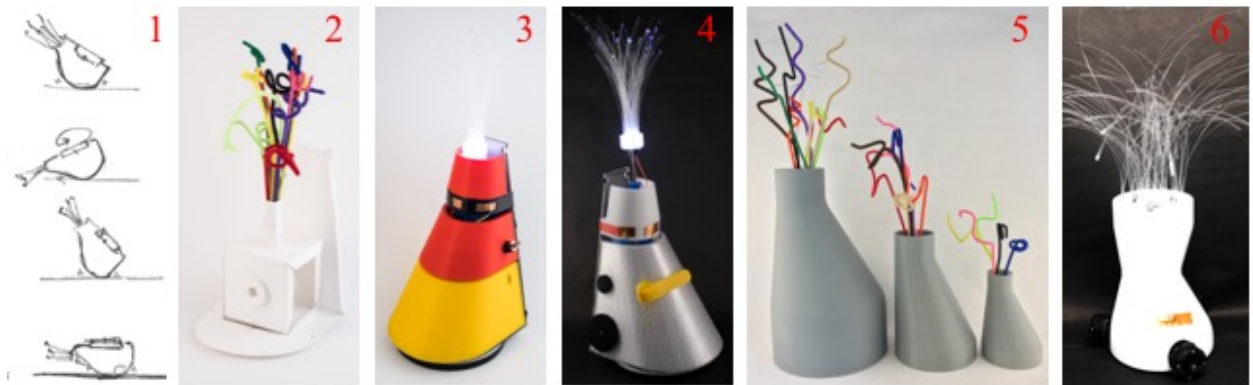
Figure 1. Iterative prototypes of the robot designed developed during the design process. Left to right: (1) early hand-ketches capturing movement analysis; (2) paper prototype to explore the size and mechanisms; (3) first actuated prototype; (4) second actuated prototype; (5) three different passive robot stand-ins for size and grasp studies; (6) final version of the robot. Retrieved from Alves-Oliveira, Arriaga, Paiva, and Hoffman (under review).
