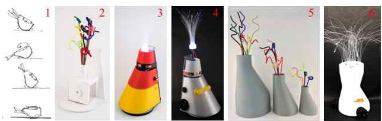
Figure 1. Iterative prototypes of the robot designed developed during the design process. Left to right: (1) early hand-ketches capturing movement analysis; (2) paper prototype to explore the size and mechanisms; (3) first actuated prototype; (4) second actuated prototype; (5) three different passive robot stand-ins for size and grasp studies; (6) final version of the robot. Retrieved from Alves-Oliveira, Arriaga, Paiva, and Hoffman (under review).
