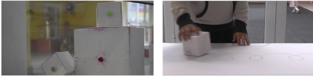
Figure 2: Left: Paper prototypes of robots used in the design condition were made using origami techniques and each cube was built with a mechanism that integrates a crayon inside so that children could represent the movements of the robot by drawing them in large paper sheets. We embed a crayon in one of the cube faces as a design methodology that motivated children to represent the robot's movements in a 2D space, avoiding movements in a 3D plane (such as flying and jumping) as real robots are not able to do so. Right: Example of a trajectory performed by a child.
