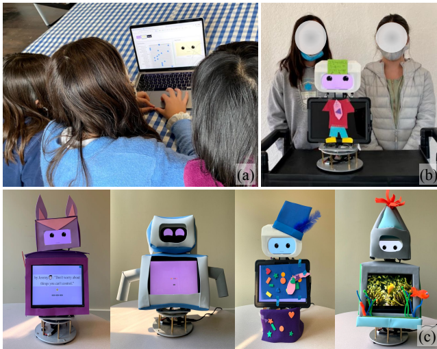
Figure 11: (a) Three children using the FaceEdit tool in FLEX-SDK to design a robot that would help them learn English as part of CS-7 and (b) two others showing their design. (c) Robot embodiment examples designed for different applications in CS-7 where participants used the FaceEdit and IOEdit tools to create the face and belly screens of their robots.
