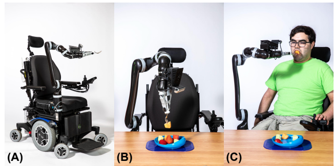
Figure 1: The robot-assisted feeding system used in this work (A) picking up food (B) and feeding it to the user (C).
